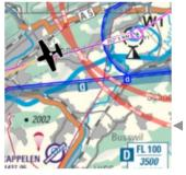
Scaled at 1.5 NM, this is how the mo ving map with SmartChart looks with an Approach Chart on overlay, a planned route, airspaces and some NOTAMs.
